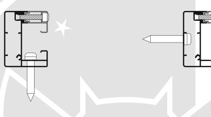
**Warning!** Make sure that the rails are screwed vertically parallel to each other; that the cassette is mounted horizontally and the diagonals between the guides are equal.
