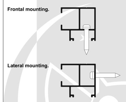
**Warning!** Make sure that the rails are screwed vertically parallel to each other; that the cassette is mounted horizontally and the diagonals between the guides are equal.
