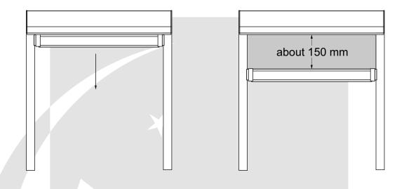
After lowering the fabric, insert it into the guiding ZIP insert and place the insert in the guide.
