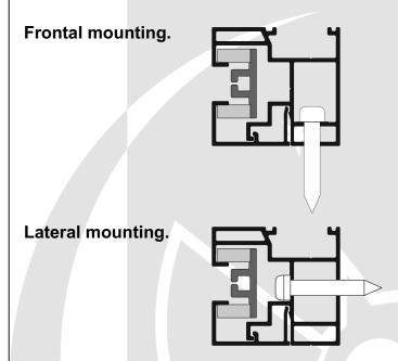
**Warning!** Make sure that the rails are screwed vertically parallel to each other; that the cassette is mounted horizontally and the diagonals between the guides are equal.
