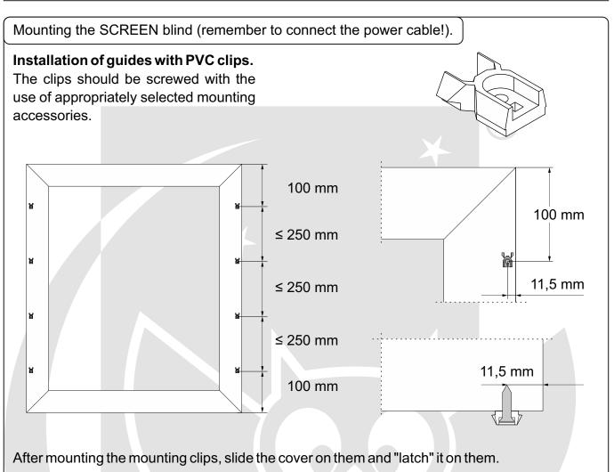
**Warning!** Make sure that the rails are screwed vertically parallel to each other; that the cassette is mounted horizontally and the diagonals between the guides are equal.
