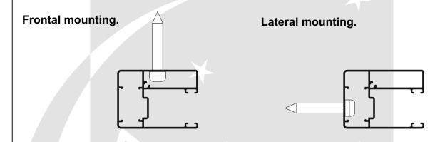
**Warning!** When screwing the guides, make sure that the rails are screwed vertically parallel to each other; that the cassette is mounted horizontally and the diagonals between the guides are equal.
